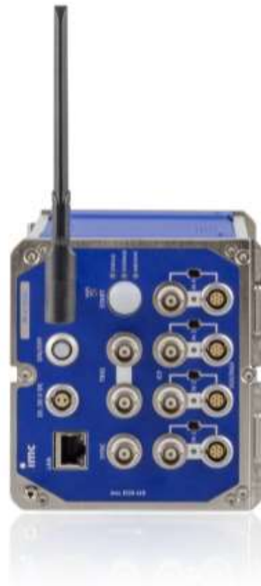
Fig. 2: imc EOS-U4 with integrated WLAN
