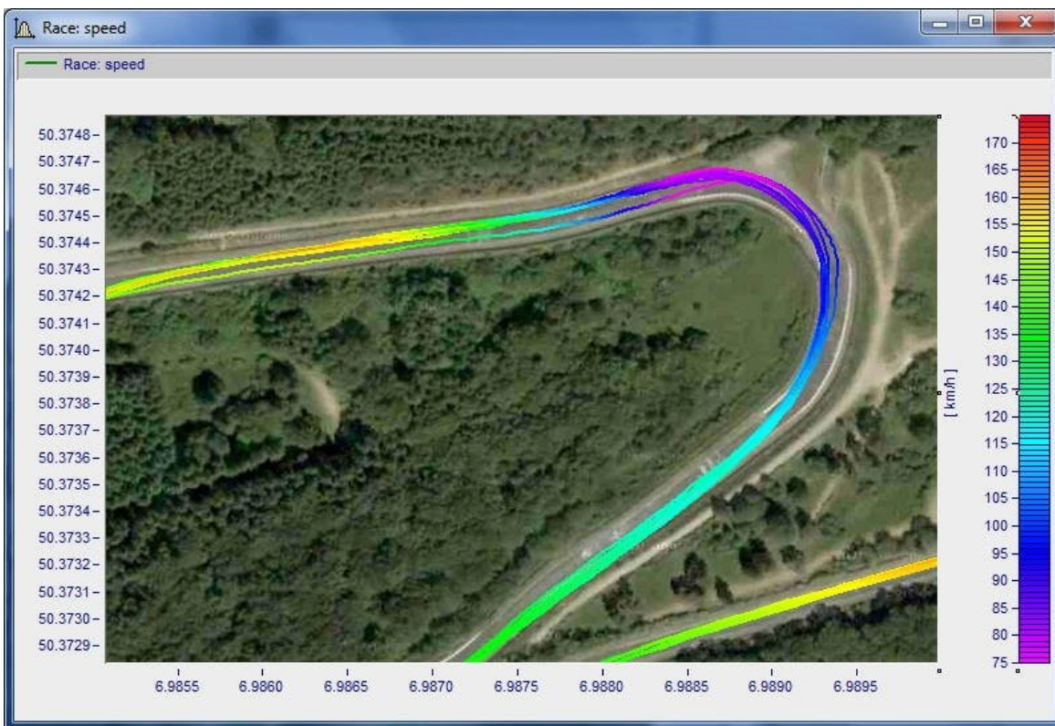
Color of position signals depending on speed
