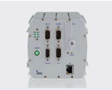
imc BUSDAQ-X, multi-bus/multi-protocol data acquisition system
