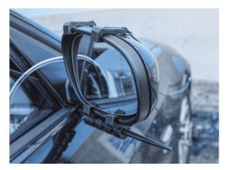
Dx-antenna for mounting on side mirror
