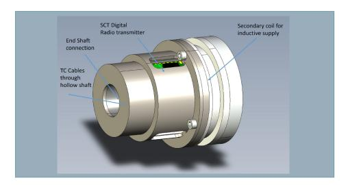
**FIGURE 4.**Rotor with imc D<sup>X</sup>
