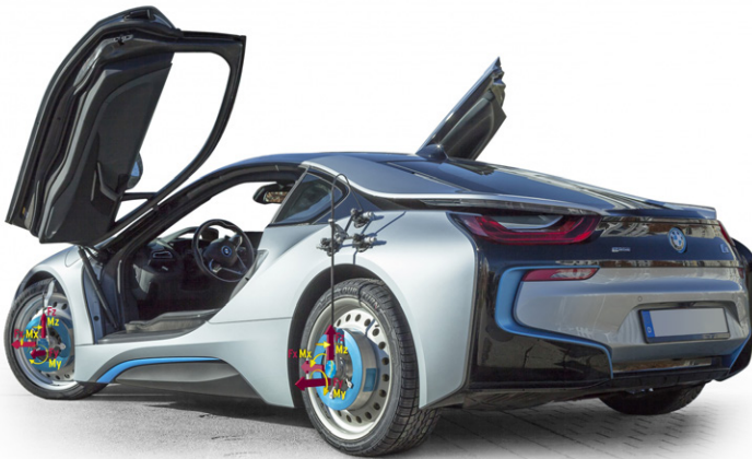
The use of measuring wheels provides information about wheel contact and lateral forces on the e-car
