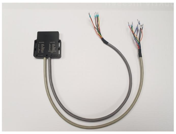
Fig. 7:  $D^{X}$ -SCT with connection cable integrated in a special housing
