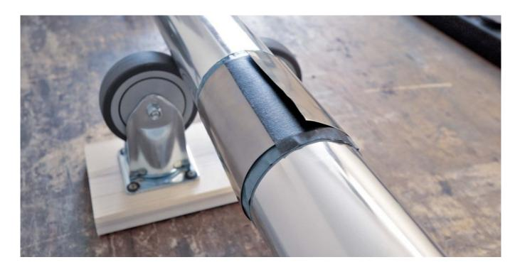
Fig. 32: After applying the second Mu metal layer
