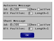
This function allows other devices to remotely activate the "Autozero" function or the "Test Shunt" on your D<sup>x</sup> system.
