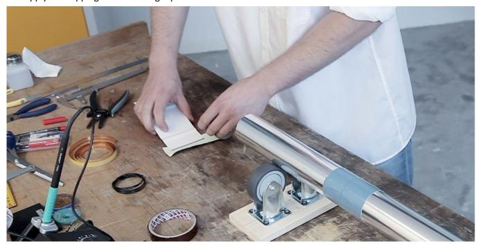
3. Pull off the protective foil and stick the Mu metal onto the shaft. The ends must not touch, there must be no short-circuit winding with the Mu metal.
