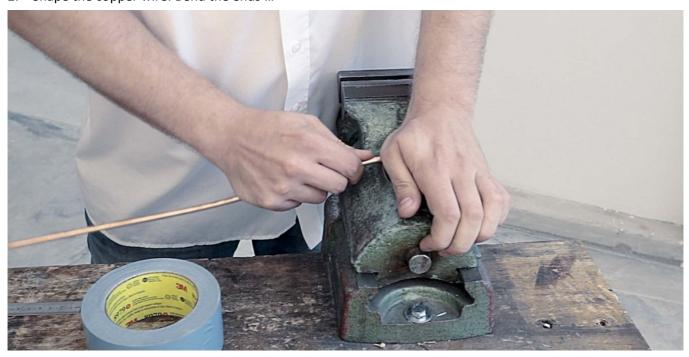
Fig. 46: Bend the ends of the copper wire
