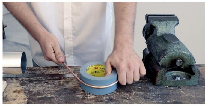
Fig. 47: Form the arc of the ring stator
