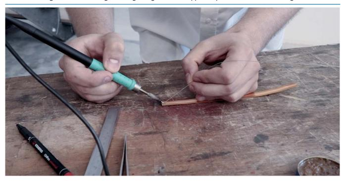
Fig. 38: Solder the wires for the inductive power supply to the copper strip.
