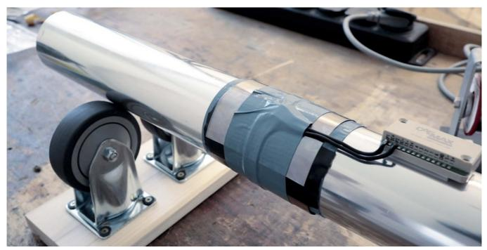
Fig. 43: The finished secondary winding
