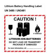
Fig. 1: Li-Ion Handling Label
