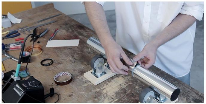
Fig. 27: Apply the first Mu metal layer to the shaft
