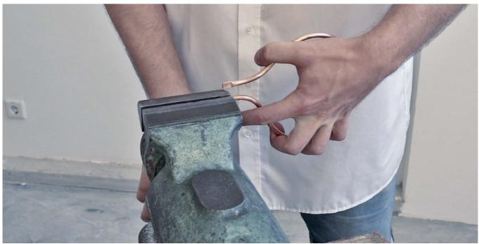
Fig. 48: Press the copper tube together at both ends
