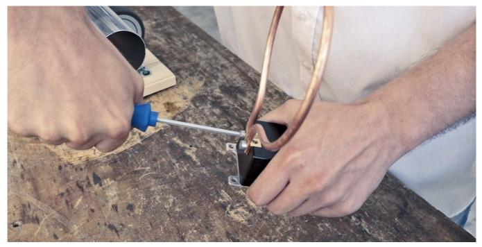
Fig. 52: Screw primary winding to ring stator
