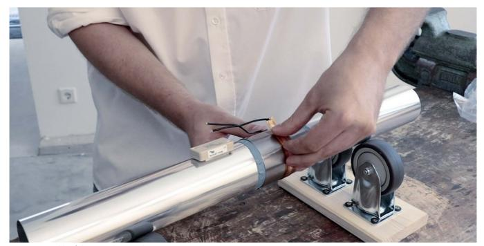
Fig. 39: Assembly of the secondary winding
