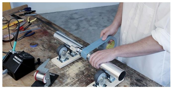
Fig. 42: Apply gray tape for isolation and protection
