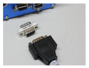
Fig. 57: CAN terminating resistor
