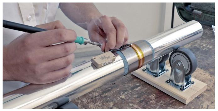
Fig. 40: Soldering the wire ends to the  $D^{X}$ -SCT transmitter unit
