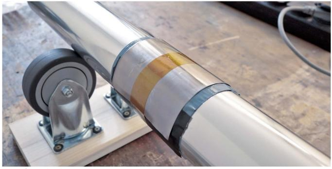
Fig. 34: After attaching the Kapton tape
