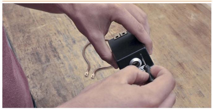
Fig. 53: Set the voltage regulator to the minimum position
