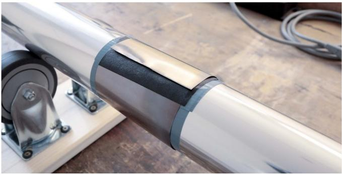
Fig. 28: After applying the first mu-metal layer
