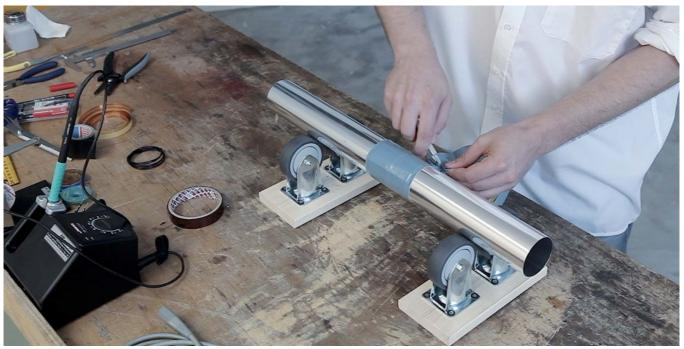
Fig. 29: Attaching isolating tape
