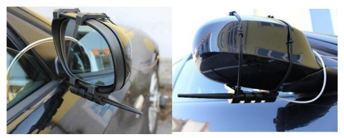
Fig. 117: D<sup>X</sup> side mirror antennas
