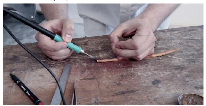
Fig. 36: Tin both ends of the copper strip
