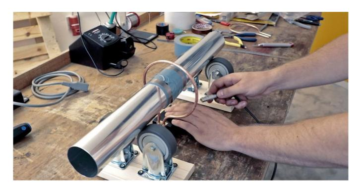
Fig. 54: Connect the power cable to the ring stator
