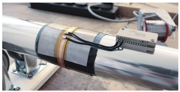
Fig. 41: Secondary winding connected to transmitter unit  $\mathsf{D}^\mathsf{X}\text{-}\mathsf{SCT}$
