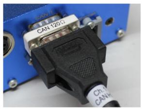
Fig. 58: Plugged CAN terminating rsistor (120  $\Omega$ )
