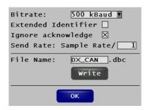
Bitrate: Setting the transmission rate for the CAN bus
