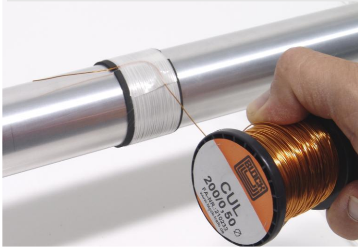
Coil, depends of shaft diameter 8-13 parallel windings of 0.5 CUL wire
