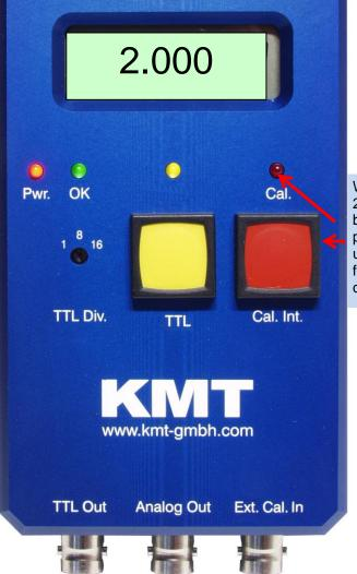
When a constant speed of 2000 rev/min is registered by the vehicle tachometer, press the Cal. Int. button until the red LED stops flashing, and remains constantly illuminated.
