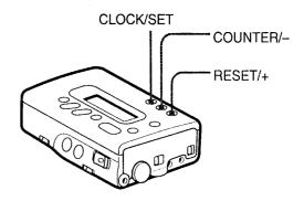
5 Press the COUNTER/- and RESET/+ buttons to set the day, then press the CLOCK/SET button.
