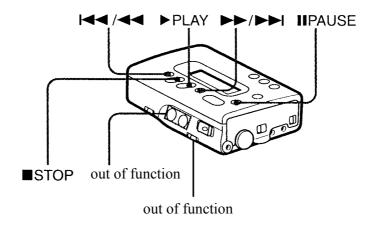
Press either  $\nearrow \nearrow / \nearrow I$  or  $I \ll / \ll$  button quickly once during playback. If the unit is in the fast forward/rewind mode, press either the  $\nearrow \nearrow / \nearrow I$  or  $I \ll / \ll$  button once. Or if the unit is in the stop mode, press either the  $\nearrow \nearrow / \nearrow I$  or  $I \ll / \ll$  button twice.
