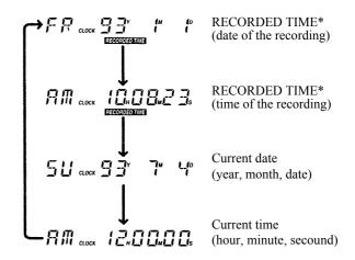
\*The RECORDED TIME will not be displayed while the unit is in the recording, recording monitor, or pause mode.
