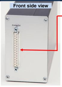
Female 37 pole Sub-D for analog signal output, CH 1 to 32
