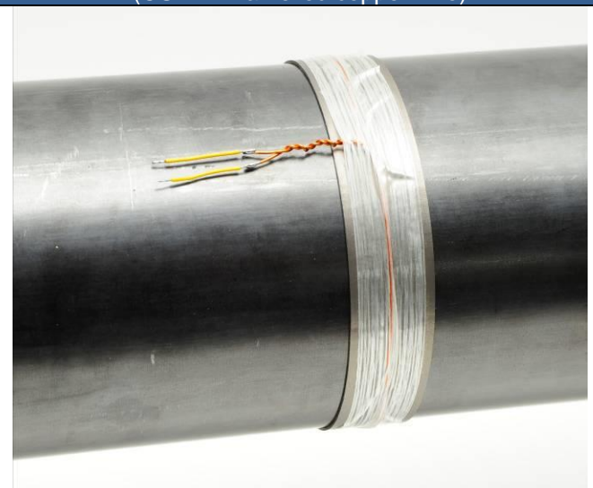
Extend the CUL wire flexible 0.14-0.25mm wire (to decouple the inflexible 1mm wire!)
