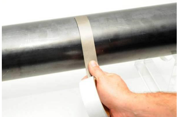
Attach for electromagnetic insulation "Ferrite Tape" 2 x one layer around the shaft.
