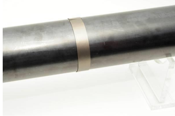
Attach for electromagnetic insulation "Ferrite Tape" 2 x one layer around the shaft.
