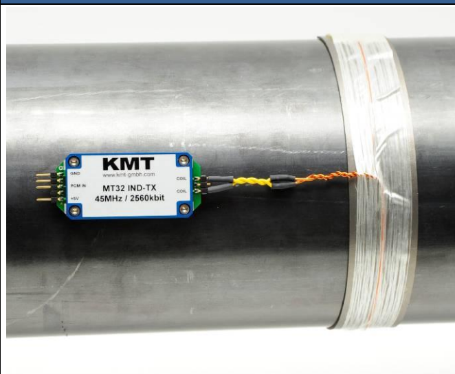
Twisted also the flexible wire and solder it on the MT32-IND-Tx (isolate all solder points with shrink tubing)
