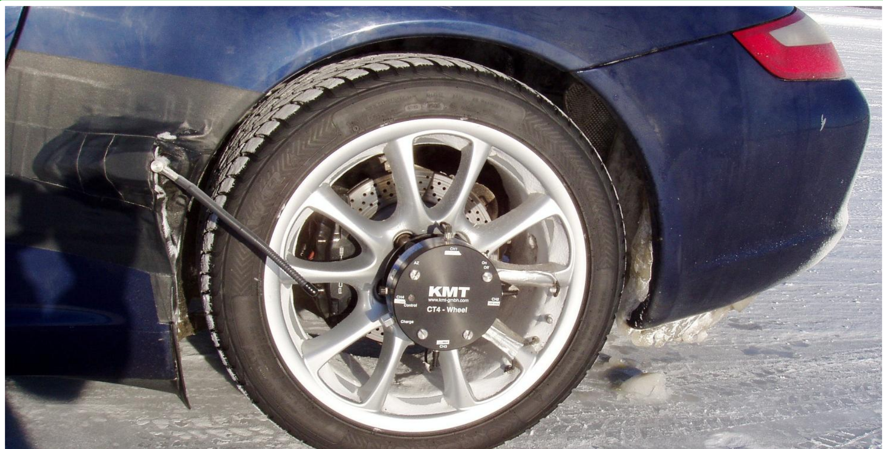
Vibration test from racing car wheel at high speed of 300km/h (Porsche)
