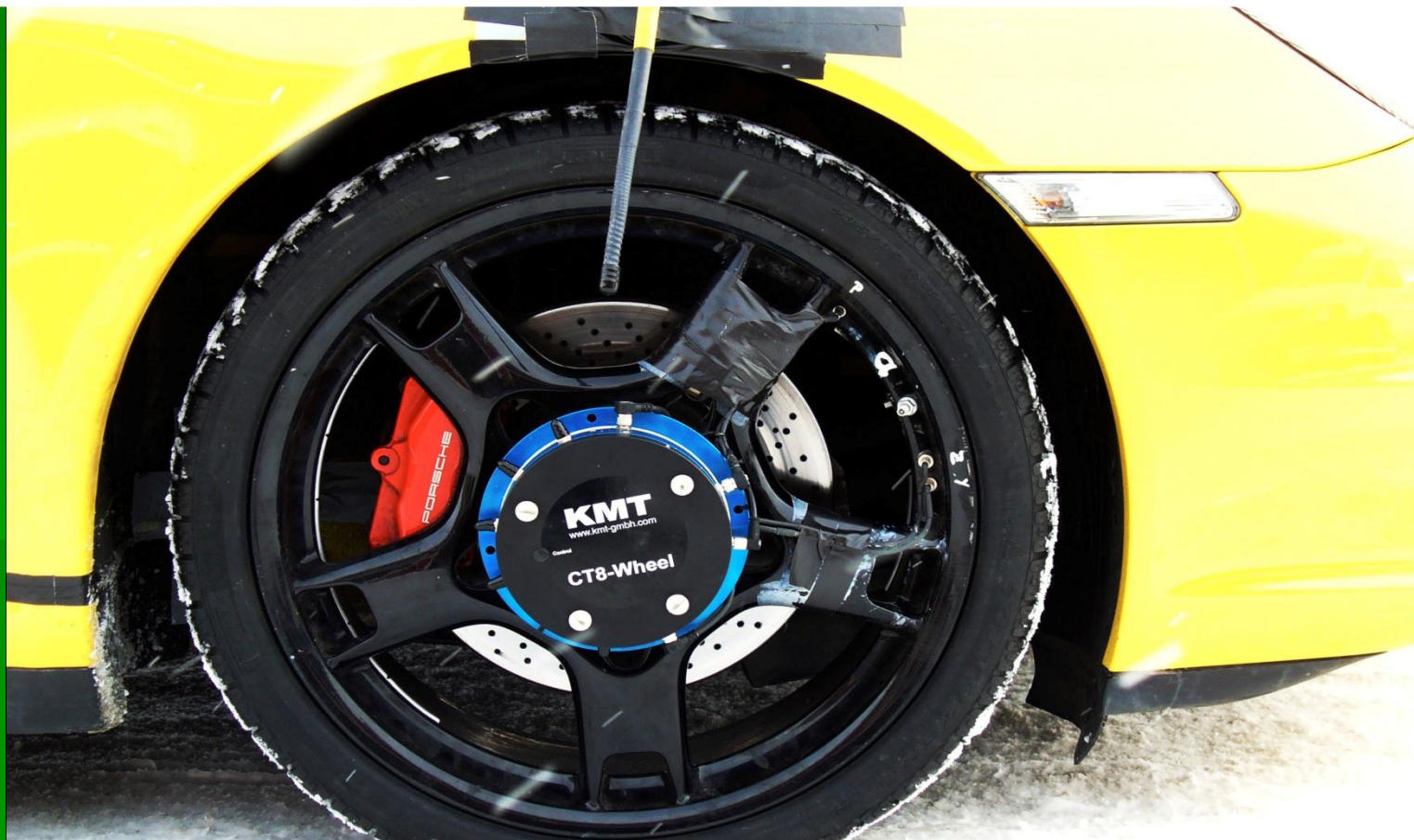
Vibration test from racing car wheel
