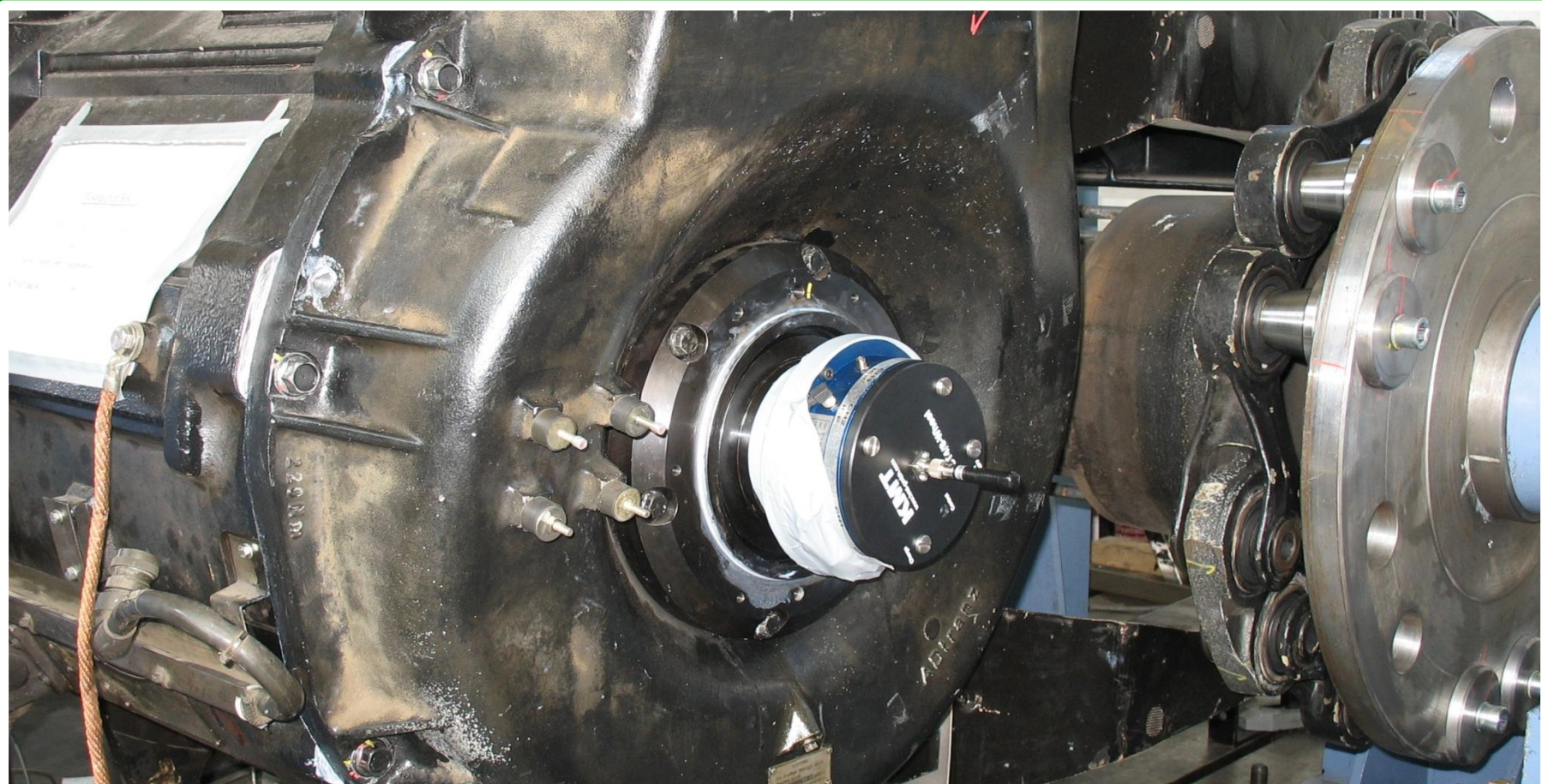
Temperature & force measurement inside of electric motor (railway)
