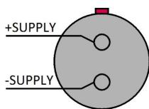
The imc CANSASflex modules can be powered by a DC supply voltage which is supplied via a 2-pole **LEMO.EGE.0B compatible socket** (multicoded 2 notches). The permissible supply voltage range is: **10 V to 50 V**.
