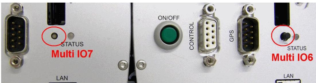
From Multi IO7 onwards, the button is countersunk, so that to press it a sharp object like a pen is needed.
