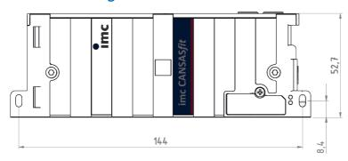
Module shown in standard operating position (terminal connections upwards)
