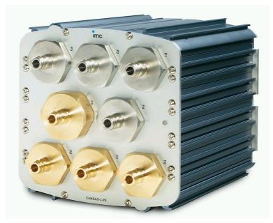
The module family CANSAS-P8, with its 8 nipples built into the housing, is designed to take measurements of pressure. A tube can be connected to these nipples via a coupling, and either the absolute or relative pressure of the gas or liquid in the tube can be measured, depending on the sensor in the nipple. A barometer inside the module makes it possible to derive the relative pressure even when using sensors for measurement of absolute pressure.
