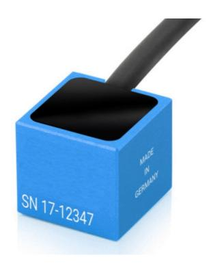
The capacitive accelerometers are based on microelectromechanical systems (MEMS technology) and allow static measurement of acceleration forces from 0 Hz upward. The scope of application possibilities includes the fields of vehicle dynamics, endurance strength testing, vehicle inspections, brake testing, driving comfort measurement, structure monitoring, or in general wherever reliable measurement of acceleration is needed.
