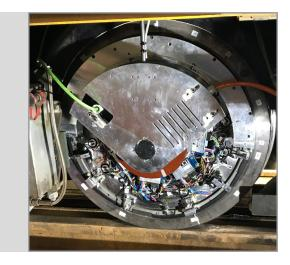
The telemetry system consisted of several components, of which 16 sensor modules were integrated into the measurement wheel and the controller module outside of the wheel, for wireless data transfer. This setup is especially suited to rotating applications and components.
