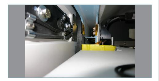
The recording of strain gauge signals requires precise and reliable measurement devices since the voltage signals to be measured are in the range of a few microvolts. imc CRONOS systems were the ideal solution. It was possible to record frequencies relevant for the measurements of up to 200 Hz and to process signals with a correspondingly high resolution.
